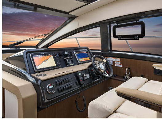
The fully equipped control station features SmartCraft™ diagnostics and VesselView display, plus a Raymarine® e125 widescreen radar/GPS/chartplotter or optional dual displays.
