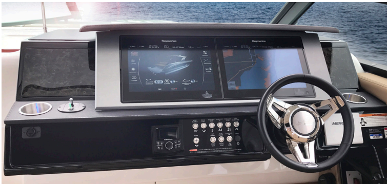
Innovative standards found throughout the SLX 400 include an advanced Digital Dash interfaced through standard twin 12" Raymarine glass displays and Axius® propulsion with joystick control for effortless docking and maneuvering in the tightest of spaces.
