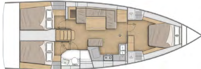
3 cabins 1 head version (+ Sink unit)
