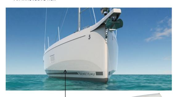
Located above the waterline, the integrated stepped hull chine increases interior space while keeping the hull performance.
