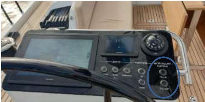
Control to fill/empty the water ballasts on each helm console
