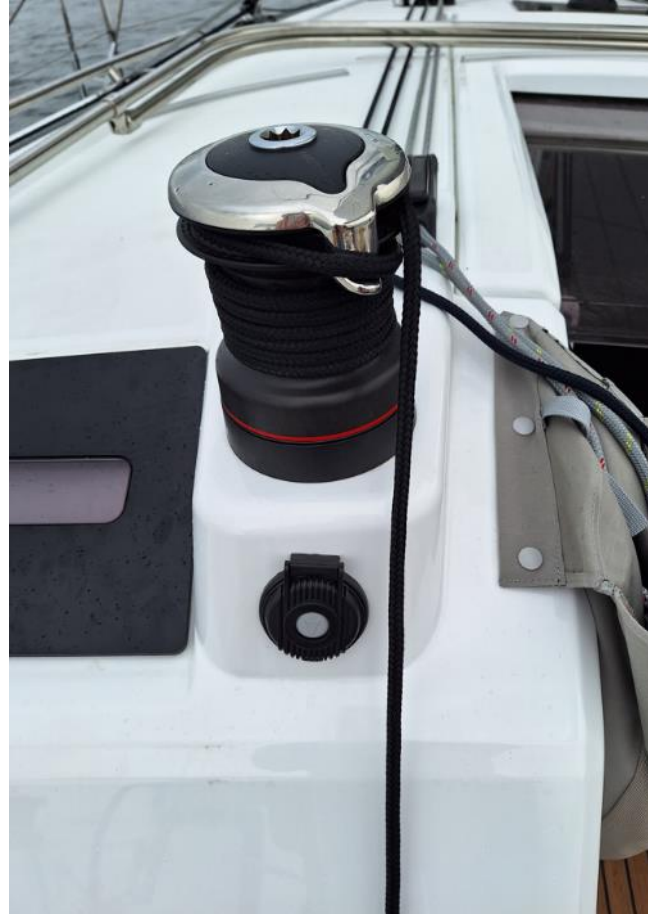
Electric winch on the port side
